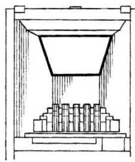
5.5 Place the front coal centrally in the channel at the front of the tray. The relationship between the front coal and flame baffle is shown in Diagram 17.
