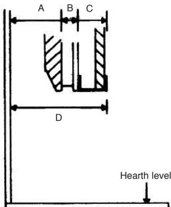
When fitting the Logic Convector fire and a Stovax Cast Iron Convector fireplace to a precast letter box flue with a standard starter block, the 8315 spacer kit will be required, together with an extra deep 142mm rebate surround.
