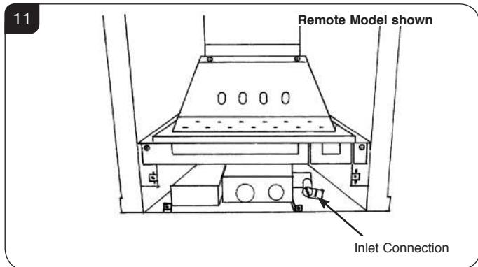
4.11 Carefully refit the burner assembly.
