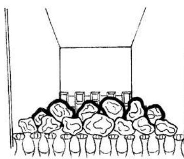
5.9 Place one small coal either side on top of the flame baffle in each rear corner. Then place two large coals in between the two small coals. These coals should touch the rear panel, see Diagram 21.
