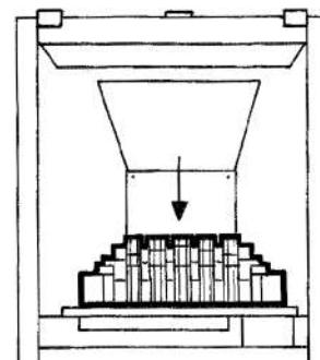
5.3 Place the rear panel against the rear of the box and slide the side panels on either side of the flame baffle. Ensure they locate in the brackets at the top of the firebox. DO NOT SLIDE THEM ALL THE WAY BACK, see Diagram 15.
