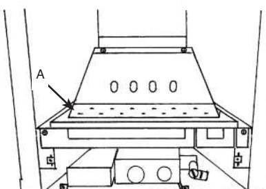
5.2 Position the flame baffle centrally on the tray and ensure the stepped lower edge engages against the rear edge of the burner skin, see Diagram 14.
