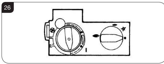
6.9 Press in the right-hand control knob and rotate anti-clockwise until a click is heard. Continue to press in. The knob points to the pilot (—).
