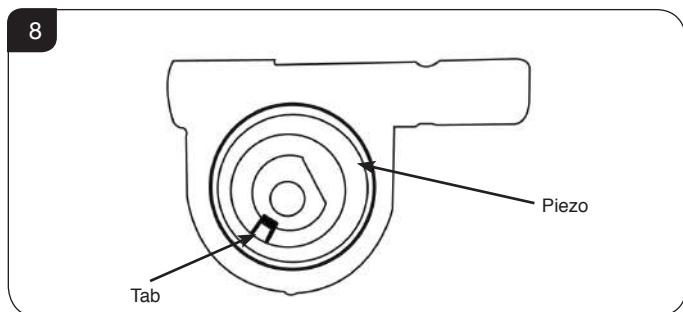
2.7 Withdraw the Piezo unit forward from the valve.
