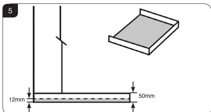
2.4 If the appliance is greater than 50mm above the floor, then no hearth is required, although due consideration should be given to how the heat may affect the floor material.
