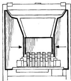
5.4 Locate the top panel on top of the rear and side panels. Finally push the sides fully towards the rear panel. This will retain the top panel, see Diagram 16.
