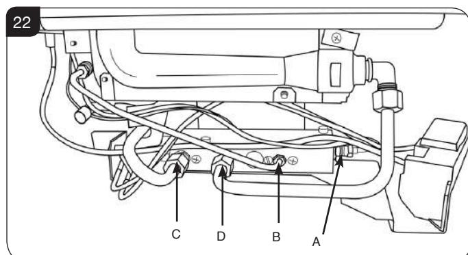
5.10 Undo the pilot pipe from the gas valve, see Diagram 22, Arrow B.
