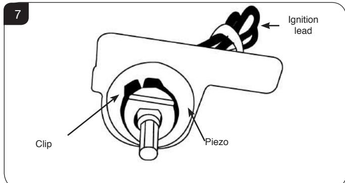
2.6 Rotate the Piezo anti-clockwise until the tab appears in the slot at the front, see Diagram 8.
