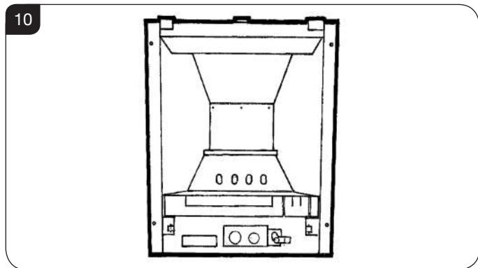
4.9 Offer the firebox into the opening and ensure that the gas supply pipe passes through the rubber seal.
