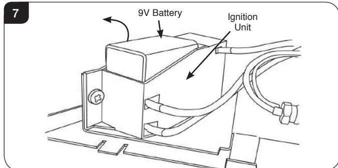
3.2 Remove the old battery and replace with a new high quality (Duracell or similar) 9V battery.
