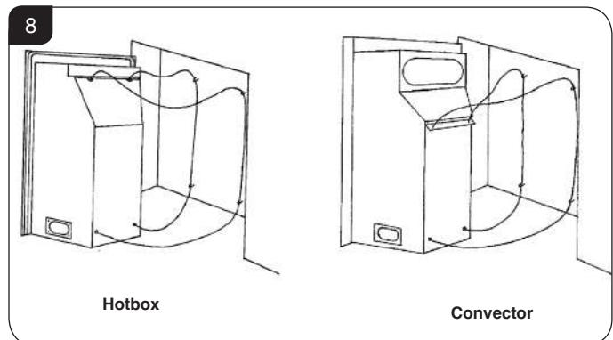
4.4 Pass the cables vertically through the 2 sets of eyebolts and thread the ends through the holes in the lower back of the firebox. Pass the gas supply pipe through the hole in the rubber seal and push the appliance into place.
