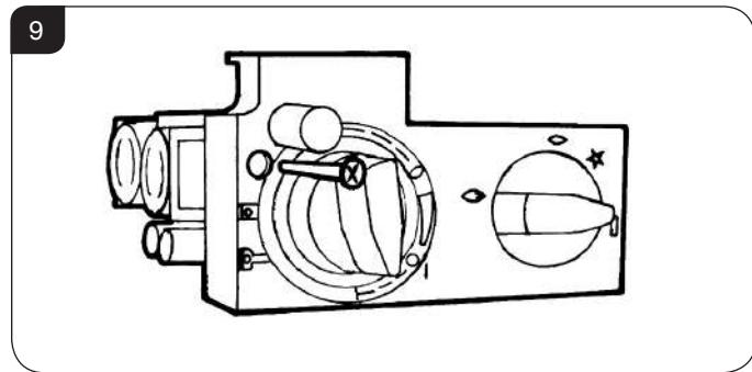
2.12 To release the right hand side of the control cover insert the narrow blade screwdriver into the slot shown in Diagram 10, lever it gently and pull from the right hand side at the same time. The cover will now come off, there is a small cylindrical metal spacer inside the cover, this must be kept and replaced on the fixing screw during re-assembly.
