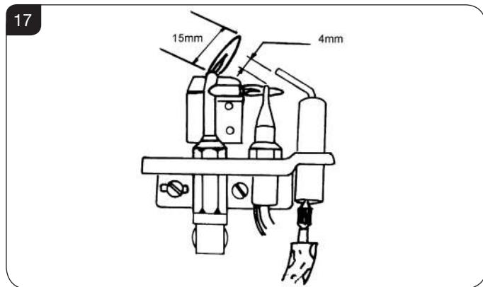
4.11 After reassembly, check for gas soundness and carry out a flame failure functional check details in the flow chart, especially the time it takes for the mag unit to close.
