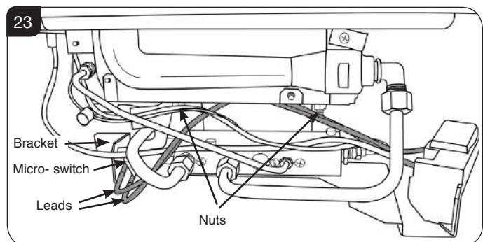
5.15 Undo the screw from the end of the spindle and remove the bracket, see Diagram 23. Ensure the **bracket is replaced during reassembly**.
