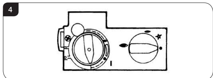
2.9 Press in the right-hand control knob and rotate anti-clockwise until a click is heard. Continue to press in. The knob points to the pilot (—).
