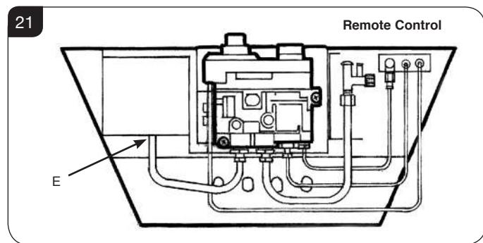
5.6 Undo the lock nut (Manual model) or 2 bolts (Remote model) securing the gas valve to the appliance and remove the valve.
