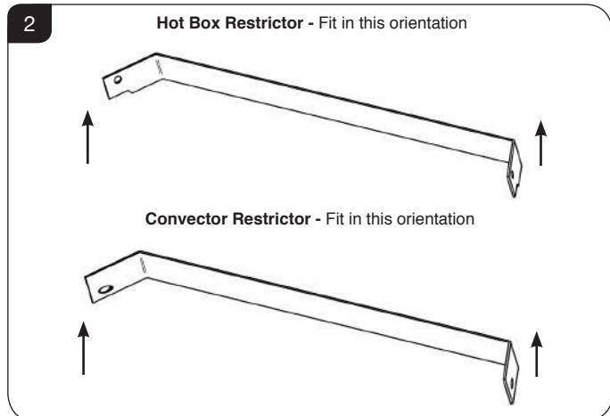
This is fitted from inside the appliance across the outlet at the top of the firebox with two screws provided, see Diagram 3.
