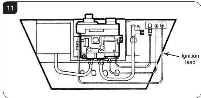
2.14 Replace with a new ignition lead following the same route as the old one. Replace the valve cover and the pilot assembly.
