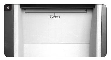
4.3 The baffle can now be removed through the front of the appliance.
