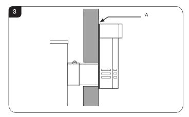
3.23 Feed the flue through the wall, making sure it runs smoothly.
