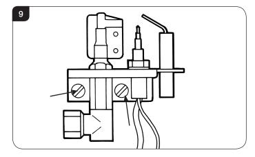
5.4 Reassemble in reverse order, do not overtighten.
