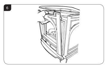
5.4 Remove the glass frame by undoing the fixing screws and lifting clear, see Diagram 7. Take care to support the glass window panel when removing the screws.
