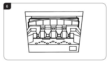
7.3 Place the coal retainer in the two guides as shown in Diagram 7.
