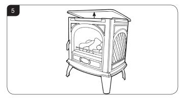
5.3 Lift the front upwards until it is clear of the slots and pull away from the appliance, see Diagram 6.
