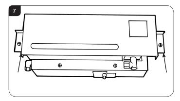
5.2 Remove the lint arrestor by folding the tabs back, see Diagram 8.
