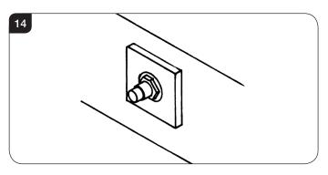
10.5 Extract the injector with the feed pipe from beneath the appliance.
