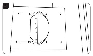
3.6 Position the flue spigot using the offset holes and the ones previously beneath the blanking plate. Secure the spigot and blanking plate in new positions, see Diagram 3.
