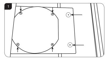
3.5 With the blanking plate removed there are two additional holes underneath, see Diagram 2.
