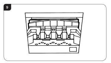
7.3 Place the coal retainer in the two guides as shown in Diagram 10.
