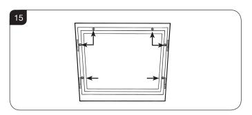
8.2 Replace ALL of the securing screws ensuring that a screw is present in all fixing slots.
