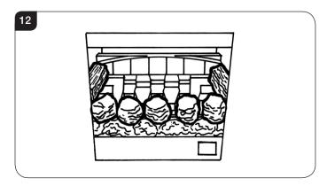
7.6 Place four of the loose round coals behind the first row so that they sit on the fingers of the flame baffle, the two outer ones should touch the rectangular coals, see Diagram 13.
