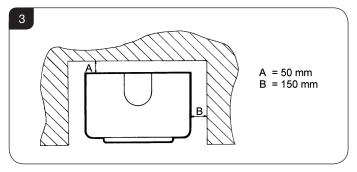
5.5 In a non-combustible recess be careful to allow enough clearance at the sides and rear of the appliance to perform spillage tests and reach the controls.
