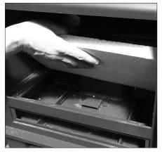
Remove the upper secondary steel baffle and internal vermiculite baffle (for further instruction please see under maintenance heading).
