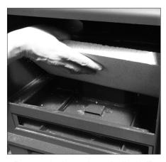
Remove the internal vermiculite baffle (for further instruction please see under maintenance heading).
