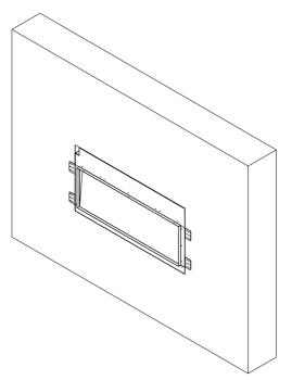
7. Using desired materials, finish to the glass for a clean face installation OR re-attach the steel surround that was removed in STEP 1.
