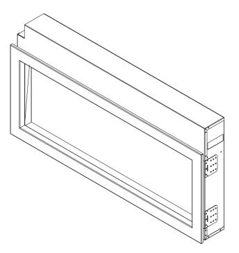
2. Remove the optional trim from the unit as illustrated below. Remove the wall framing plates from the unit.
