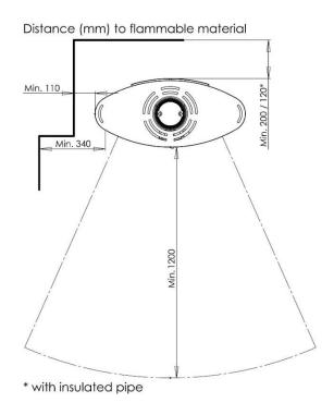
If the stove is positioned against a brick wall or other non-flammable material, there are no minimum distance requirements. To facilitate cleaning and for the best use of the convection air, we recommend that you leave a distance of approximately 5-10 cm to the wall.
