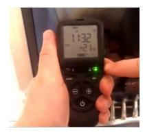
Hold the handset as shown, wrapping your hand around the handset touching both sides, and the green unlock light will illuminate allowing the buttons to work.
