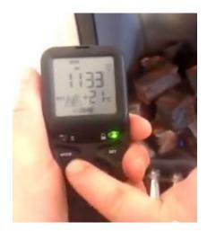
To adjust the flame, hold the handset to enable the buttons to work and press and hold the - button to reduce the flame. Tapping the button will adjust the flame step by step. Holding the button will skip through the steps.
