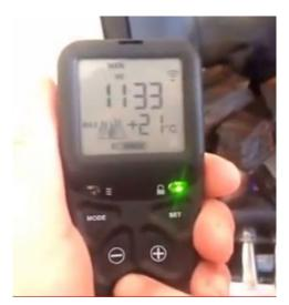
To STOP the fire, hold handset to unlock the buttons and then press the power button. The fire will stop without delay. Wait for the word OFF to appear on the display (LH Side) before trying to start again.
