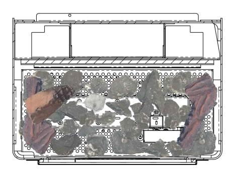
Position Log 3 (Inverted in position to log 2, as shown).
