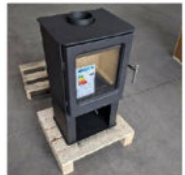
Align the base with the stove body and reinstall the retention bolts - first only finger tight to allow the base to be re-positioned to perfectly align the base before finally tightening them with a socket wrench.
