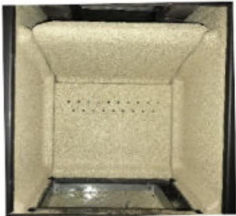
Place hand through ashpan and lift the cast iron grate up and remove from stove.
