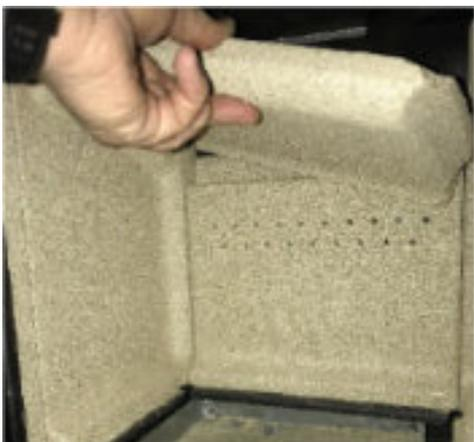
Remove Baffle brick by lifting up brick and sliding forward , then tilt brick slightly to remove.
