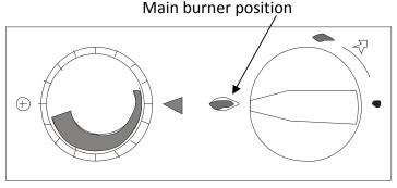
Main burner operational & thermostatically controlled
