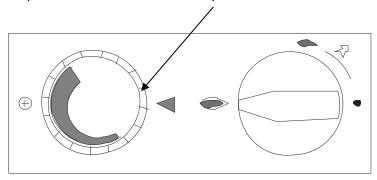
1.7. To turn the fire off, rotate the right-hand knob fully clockwise back to its OFF position.
