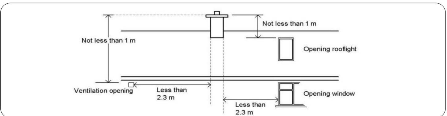
The outlet of a chimney or flue pipe should also be not less than 1m above the top of any opening skylight, opening window or wall ventilator within 2.3m
