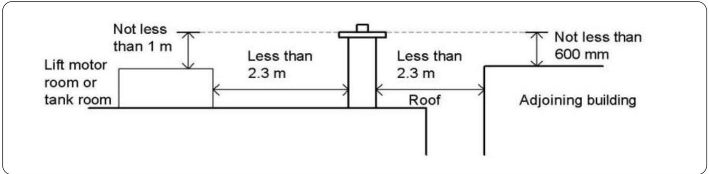
The Outlet of a chimney or flue in relation to an adjacent building should be as seen above
