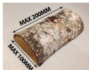
Wood length max 200mm, and 100mm in diameter.
