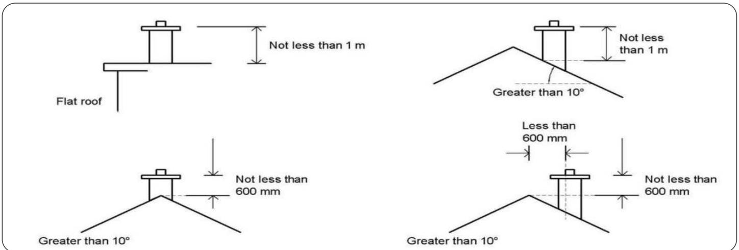
Outlet of a chimney or a flue to be not less that 1m above the highest point of contact of chimney and roof. Where the roof has a pitch of more than 10° on both sides and the outlet is at the ridge or within 600mm of it, the height of the chimney or flue pipe may be reduced to 600mm.
