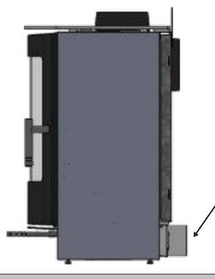
The stove requires a permanent air vent to the room. This is to provide adequate air supply in order for the stove to operate safely and efficiently. In accordance with current Building Regulations the installer may have fitted a permanent air supply vent into the room in which the stove is installed to provide combustion air. This air vent should not under any circumstances be shut off or sealed.
