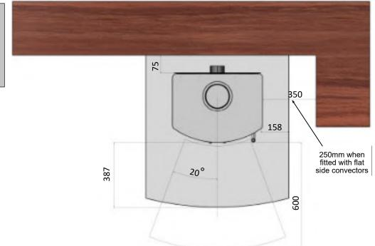
A DIAGRAM TO ILLUSTRATE THE MINIMUM DISTANCE TO COMBUSTIBLE MATERIALS
