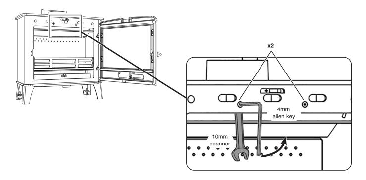
Loosen the hex bolt until the slider moves with no resistance. Once happy with the sliding action tighten the 2 locknuts.
