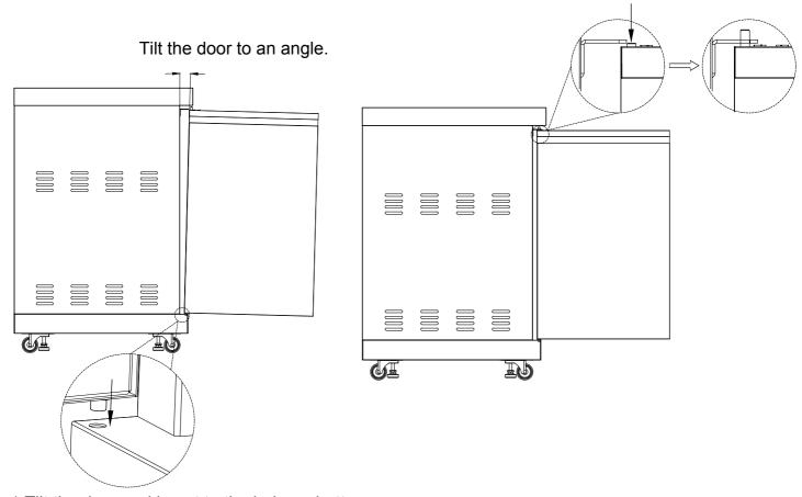
1. Tilt the door and insert to the hole on bottom.
