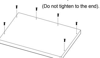
2. Position the pre-installed Screws on the cabinet (Handle with care) .
