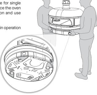
Never attempt to move the oven on your own. Two people should pick up the oven lifting from under the rounded ends of the oven, do not use the mouth of the oven as a lifting point.
