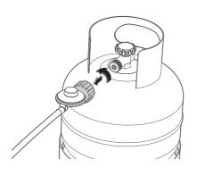
After cooking, be sure to turn off the gas from the gas canister first before turning of the Dome S1. This will allow any gas left in the burner or pipe to be used up safely. Three minutes after turning the gas off it will be safe to remove the regulator and turn the control dial back to the off position.
