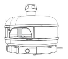
Remove the door and the stone retention wedges before lighting the oven. Do not use the door with gas burner. To light the gas burner press the control knob in and turn the knob 90° until you hear a clicking sound and the burner ignites.
