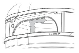
The flame should be yellow in colour and roll along the top of the oven.
