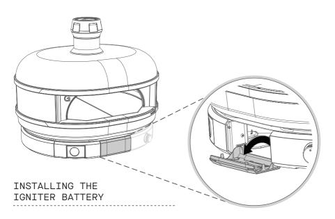
Before using the gas burner for the first time you'll need to install an AAA battery into the ignition module. To do this open the front hatch, the module will be inside and to the left. The module is held in place by a magnet, detach the module and pull it to the front hatch before unnscrewing the cap and placing the battery in (negative end first). Return the module to its original position, close the front hatch and you're ready to connect the gas bottle to the oven.
