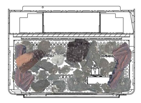
Position Log 4 as shown above, centrally at the rear of the burner.
