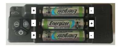
The remote display handset also has batteries as shown below. Again, remove the rear cover and replace the batteries (2 No. AA/1.5V LR6), observing the correct position as shown.
