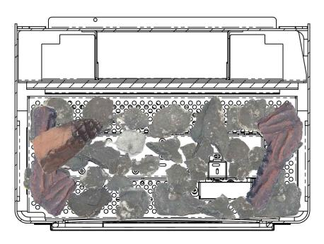
Position Log 3 (Inverted in position to log 2, as shown above).
