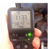
To adjust high and low whilst holding the handset and green light on press + & - to adjust for the preferred heat setting.
