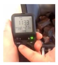
To adjust the flame, hold the handset to enable the buttons to work and press and hold the - button to reduce the flame. Tapping the button will adjust the flame step by step. Holding the button will skip through the steps.
