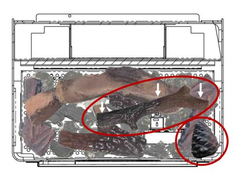
Position Log 7 as shown above. Note, this log sits on top of Log 6, Log 5 & Log 3 as shown with the arrows.
