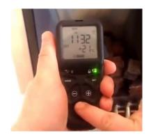
Press and hold in the power symbol button and release immediately as soon as the word pilot appears at the bottom left of the display (After about 1-2 seconds). The fire will then light onto MAX burner setting.
