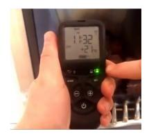
Hold the handset as shown, wrapping your hand around the handset touching both sides. In a second or less the green unlock light will illuminate, allowing the buttons to work when pushed. (NOTE: If the green light is not a constant green or not lit at all the buttons will not be operable).
