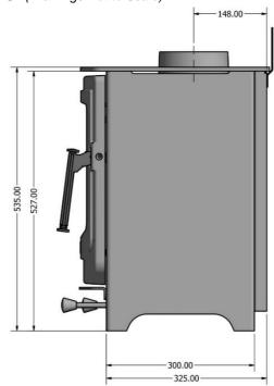
**Side View** (Showing Rear Flue Heat Shield Fitted)
