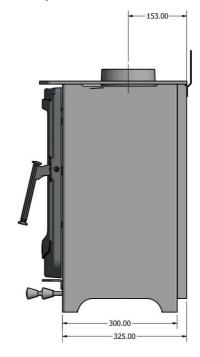
Side View (Showing Rear Flue Heat Shield Fitted)
