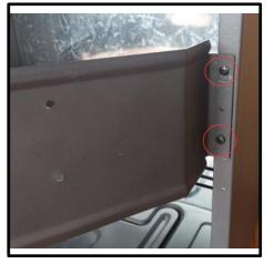
4. Align the remaining holes of the strap and heater. Proceed to place and screw 2 x screws into these holes. Completed assembly pictured above.
