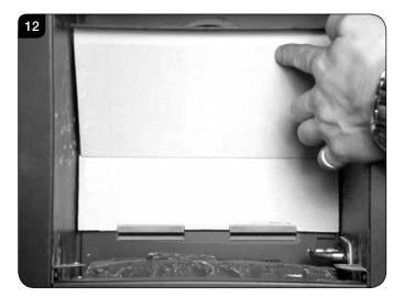
4.11 The lower rear liner does not need to be removed from the bracket in order to access the burner tray for maintenance, but can be lifted off in order to clean or replace, see Diagram 13.
