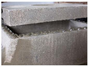
Apply lip glue to the top of the gather unit and then press the top plate into position with the hole offset closer to the rear section of the gather. Ensure the top section is level. Clean off any excess glue
