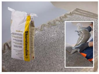
Mix lip glue jointing adhesive as per instructions on the bag. Apply 15-20mm beads using the supplied application bag as shown in the picture above.
