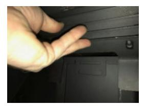
To remove rear steel baffle simply push this away from the holding frame, which it rests on, and twist it to fit through the opening.
