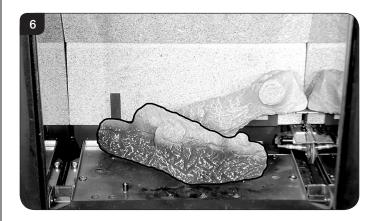
7.4 Place Log E onto the stud and behind the tag on the left hand side of the burner tray.Rest against Log B, see Diagram 7.
