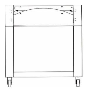
Attach the stand bar to the front of stand with 8 x M6\*12 screws.
