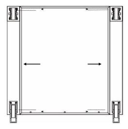
Attach the stand back plate to step 2 part with 11 x M6\*12 screws.
