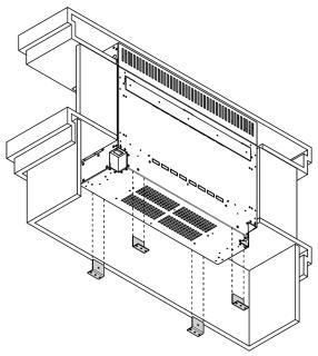
Determine the finished height and position that you want the appliance to be located. Build your base support taking into consideration the 50mm ventilation gap under the appliance. Then place the appliance onto the support and check that it is well supported.
