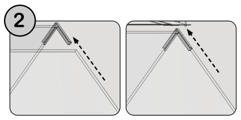
Line up the glass with the glass clip, and carefully push into place.
