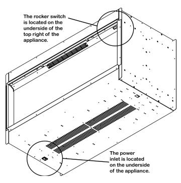
We recommend turning on the appliance before installation, connect the appliance to a power source using the provided electrical lead, and depress the right side of the rocker switch.
