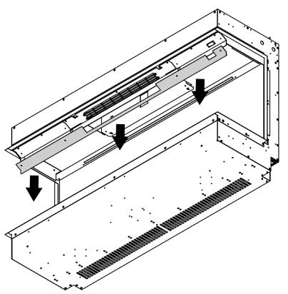
Apply the Suction Lifter to the glass and place the bottom edge in first, then angle the top edge into the appliance. Then replace the top retainer panel.
