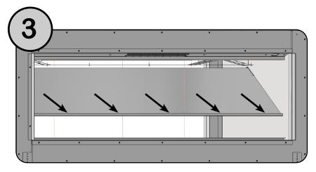
Once the glass has been inserted into the clip, ensure the bottom of the glass been fitted to rest on the retainer bar. You can then repeat the process on the other side.
