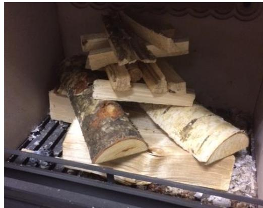
Next add plenty of dry kindling sticks and a firelighter ON TOP of the 4 logs as shown. A crib lattice pattern tends to work well. If using Maxibrite, place a layer of Maxibrite into the firebox on the base as well and omit the large logs but use plenty of kindling. Move the active baffle lever (if fitted) into the IGNITION or OPEN position.
