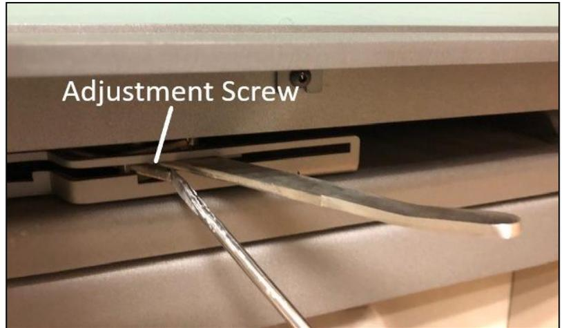
towards the user. Screwing the rod adjuster outwards (counterclockwise) causes the baffle to close further when the stove door is closed. Screwing the rod adjuster inwards (clockwise) causes the mechanism to become shorter thereby pushing the baffle less distance when the door is closed.
