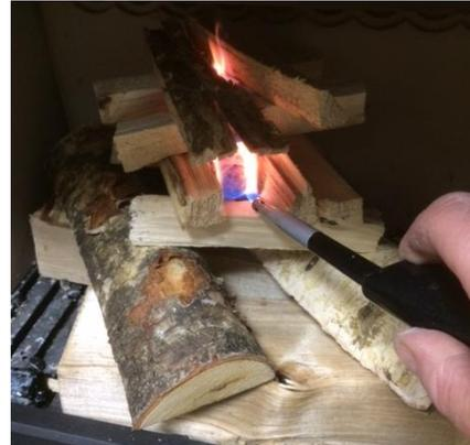
Light the firelighter(s), leaving the air control fully open and close the door. It should not be necessary to leave the door open but DO NOT leave the stove unattended if you find it necessary to leave the door ajar.
