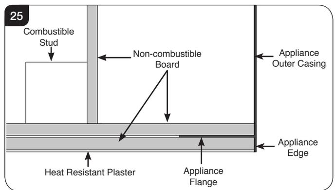
NOTE: If metal studwork is used, there is no need to fit non-combustible board to the face of the construction, see Diagram 26.
