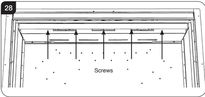
7.2 The Baffle can now be removed by lowering the front edge and pulling forward through the front of the appliance. **TAKE CARE NOT TO DAMAGE THE SIDE PANELS.**
