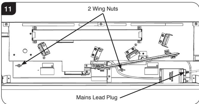
4.12 Undo the 2 wing nuts, see Diagram 11.
