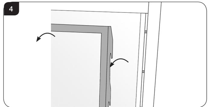
**When refitting the glass frame ensure that the rope seal on the back of the frame is intact.**
