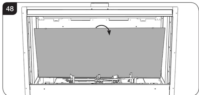
18.8 To replace the Liners and Baffle reverse these procedures. Ensure no amber glass or black shale has fallen onto the Liner Support Brackets.
