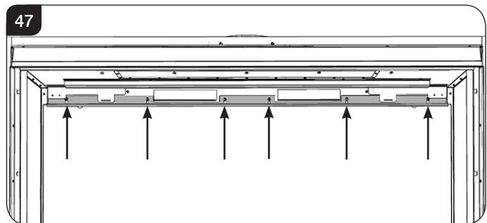
18.7 move the liner forwards off the bracket and lower into the space below.
