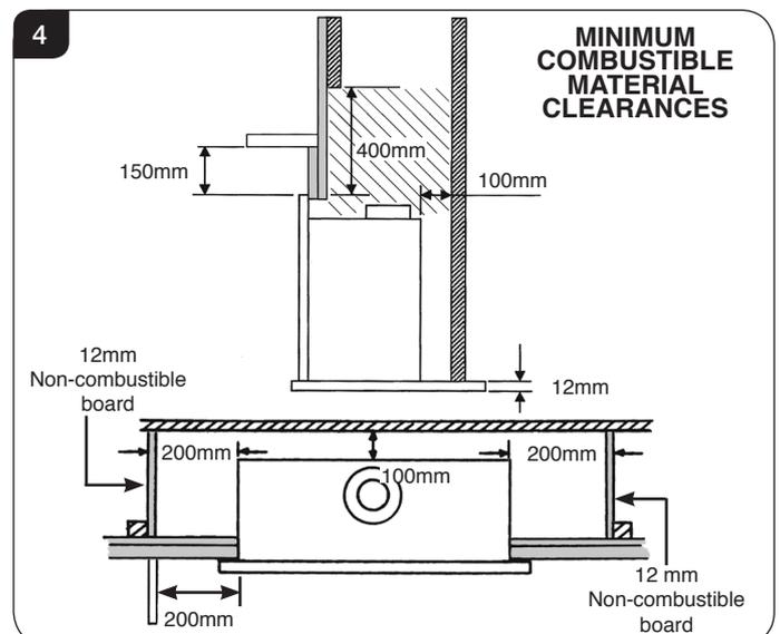
It is recommended that a marble slip or similar material is used when fitting cassette fireplaces into a plastered surface, in order to allow for heat dissipation. Also allow adequate time for newly plastered areas to dry out. Rapid drying can create cracks. In doubt, seek the advice of a professional plasterer.
