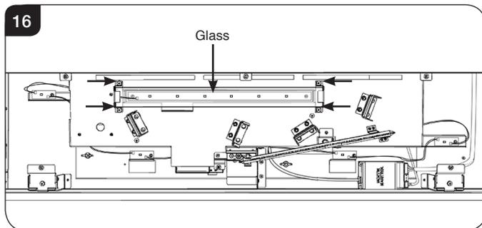
Remove the glass out of the left hand bracket and place on a dry, clean surface.
