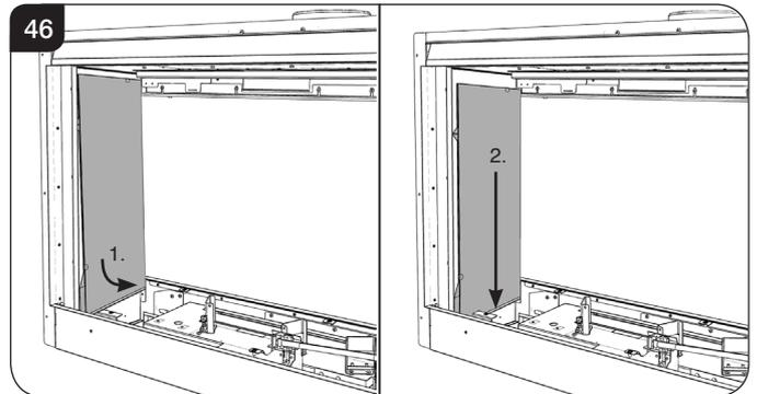
18.5 Carefully manoeuvre the side liner out of the appliance.
