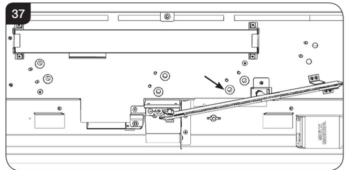
13.5 Replace with the correct size Injector.
