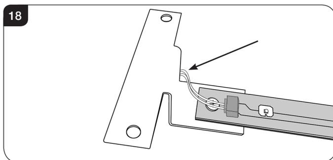
**ENSURE NO WIRES ARE TRAPPED WHEN REPLACING THE COMPONENTS.**
