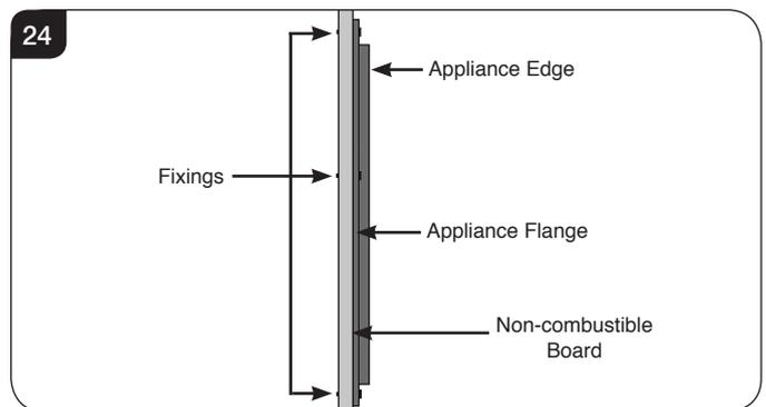
6a.12 Fit non-combustible board to the board around the appliance, see Diagram 25. Ensure distances to combustibles are observed, see Diagram 16.
