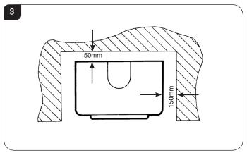
5.4 In a non-combustible recess be careful to allow enough clearance at the sides and rear of the appliance to perform spillage tests and reach the controls.
