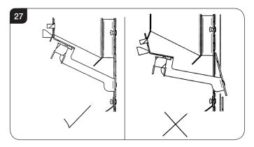
11.10 Replace the metal panel. There are spacers on the top edge to ensure the correct distance from the baffle.
