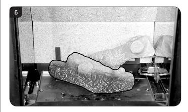
7.4 Place Log E onto the stud and behind the tag on the left hand side of the burner tray.Rest against Log B, see Diagram 7.
