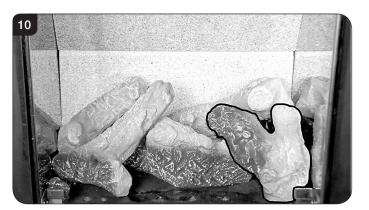
7.8 Sparingly spread an amount of the Embaglow fibres provided, covering the ports in the burner tray. Use a small piece in front of the log on the left hand side and a long strip in front of log B, see Diagram 11.
