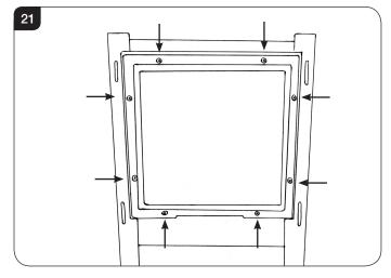
7.19 Locate the door on the 4 slots and secure to the firebox, see Diagram 22.
