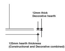
If installed at a height above 600mm from the floor there is no need for a constructional hearth in front of the appliance.
