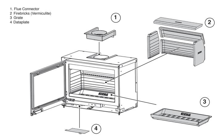
To make the installation of the appliance easier it is best to remove the internal components before fitting into the builders opening/studwork.
