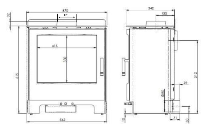
The **direct air intake spigot** (80mm diameter) to the rear of the stove is removable with a 2.5mm Allen key.
