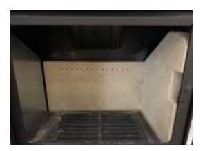
It is now possible to remove the top baffle brick by lifting up the left side and sliding it to the left then dropping it down.
