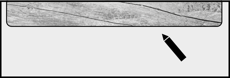
Mark bottom of beam in desired position.
